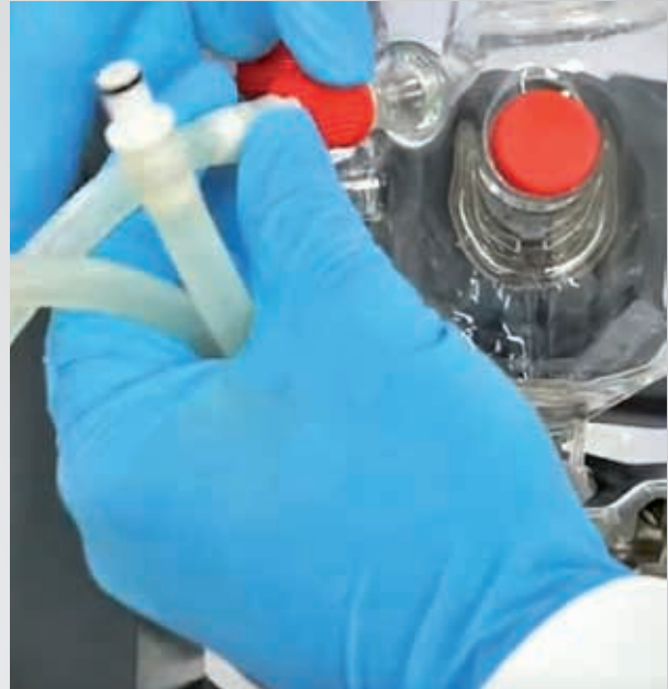
2. Connect the hoses to the rotary evaporator
