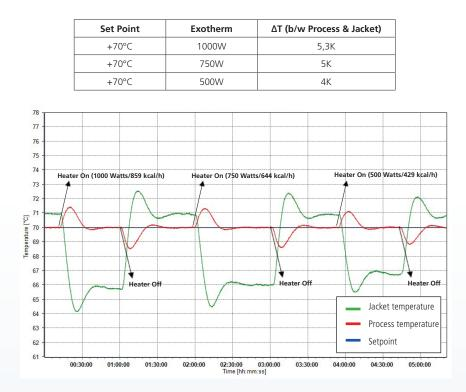
Temperature control between +20°C and +80°C, the compressor mode was selected to automatic.
