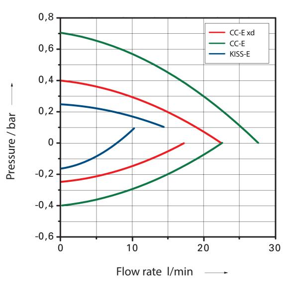
According to DIN 12876 with water at  $\,20^{\circ}\,C$
